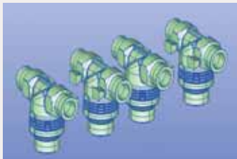
Part layout for main tree design, production rate is the main factor to be considered at this stage.
