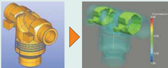
Re-analysis of the casting with predicted in-gate to resize the in-gate dimension
