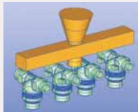
"Smart Design" knowledge base helps select the optimized casting system.
